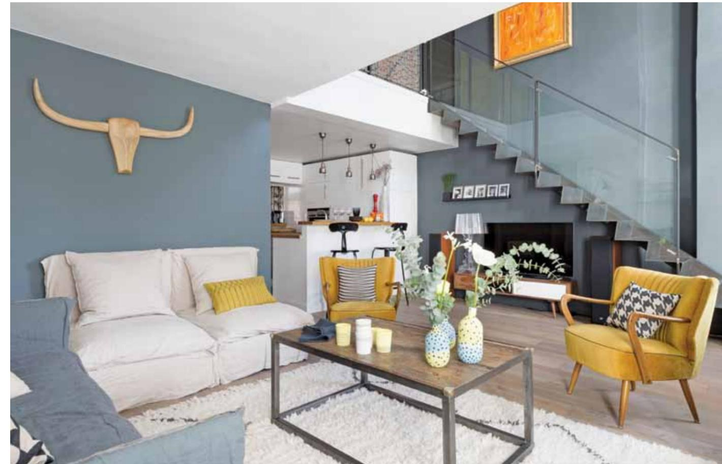
**above** The steel staircase was fabricated in Paris out of a single sheet of metal
